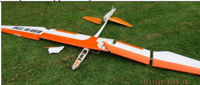
Nigel Grace's bird of time stopped flying at 600ft when half the wing fell off.
